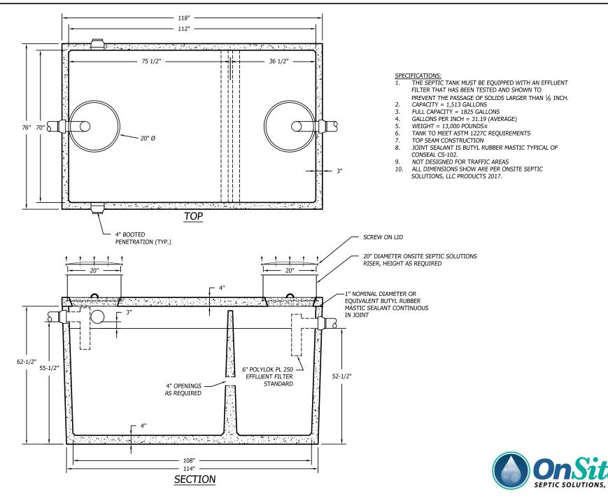
1,500 GALLON (2 COMPARTMENT) TOP SEAM HEAVY DUTY PRECAST CONCRETE SEPTIC TANK
